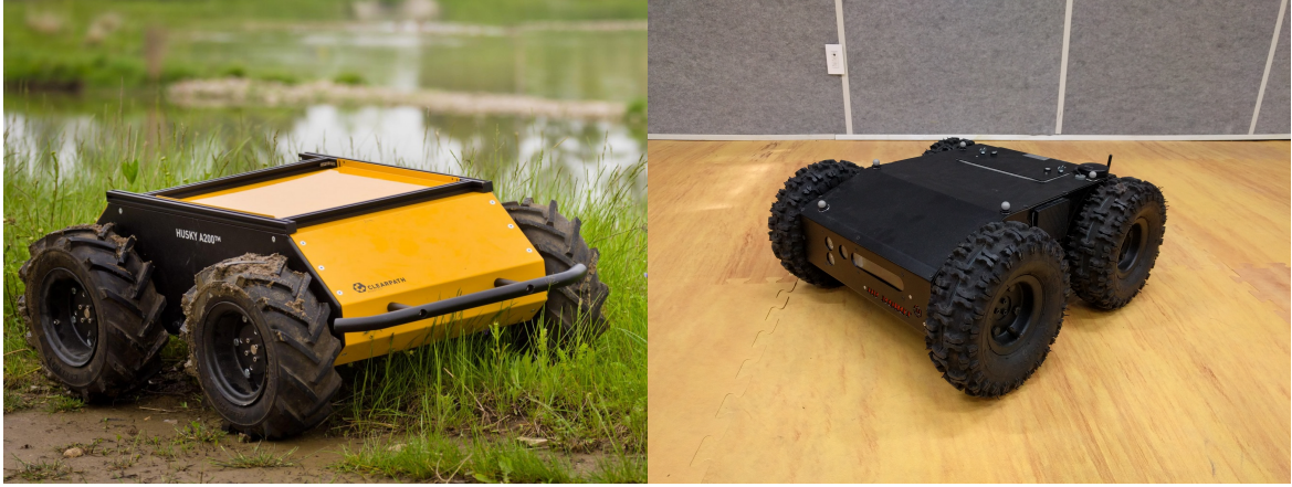
Figure 1.1: Examples of skid-steer mobile robot platform: Clearpath Robotics Husky A200 and Dr. Robot Jaguar.
