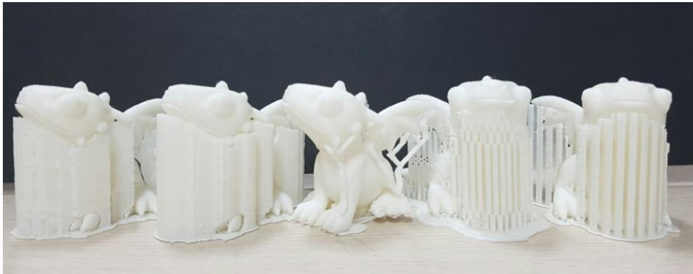
Figure 30. Cura™'s line, grid, Meshmixer's tree, Simplify3D, and Our algorithm (from left to right)
