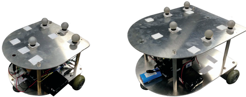
FIGURE 5.18: Small and large WMRs with VICON ® motion capture system markers used in the experiments.
