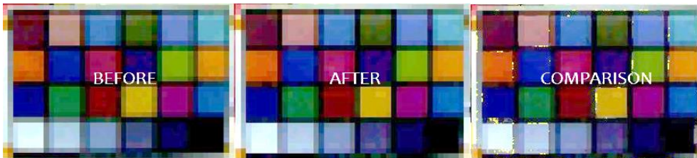
Figure 41 Shows cropped image of the ColorChecker Chart for image taken before and after the test. The third picture is the result of the comparative analysis done between the two images.
