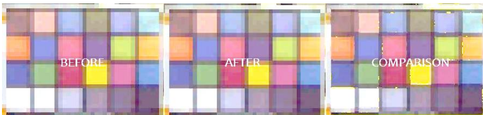
Figure 39 Shows cropped image of the ColorChecker Chart for image taken before and after the test. The third picture is the result of the comparative analysis done between the two images.
