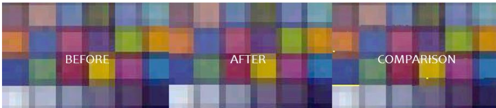
Figure 48 Shows cropped image of the ColorChecker Chart for image taken before and after the test. The third picture is the result of the comparative analysis done between the two images.
