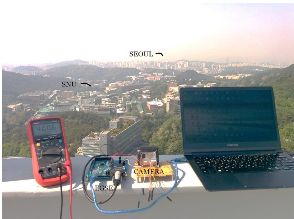
Figure 23 Outdoor testing on building 301 at Seoul National University (SNU) at Gwanak Campus. Testing equipment included EGSE, IFCAM and laptop.
