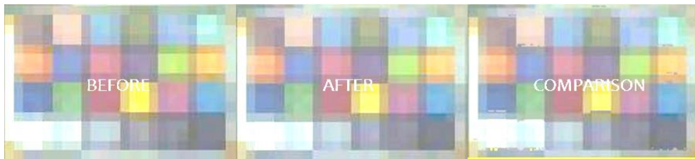
Figure 43 Shows cropped image of the ColorChecker Chart for image taken before and after the test. The third picture is the result of the comparative analysis done between the two images.
