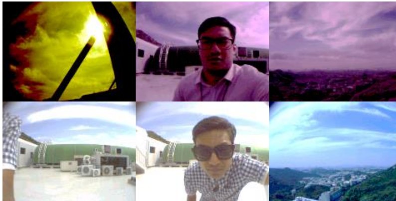
Figure 52 Comparative image between images without IR filter (top) and with IR filter (bot)
