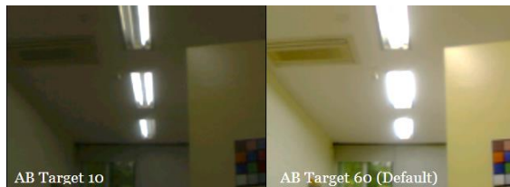
Figure 50 Another Auto Brightness (AB) or AE comparison between relative EV -2.6 and EV 0
