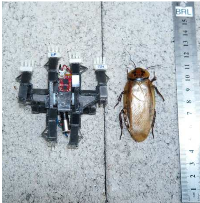
Figure 4.3 Fabrication result of the robot. Size comparison between the robot and a cockroach.
