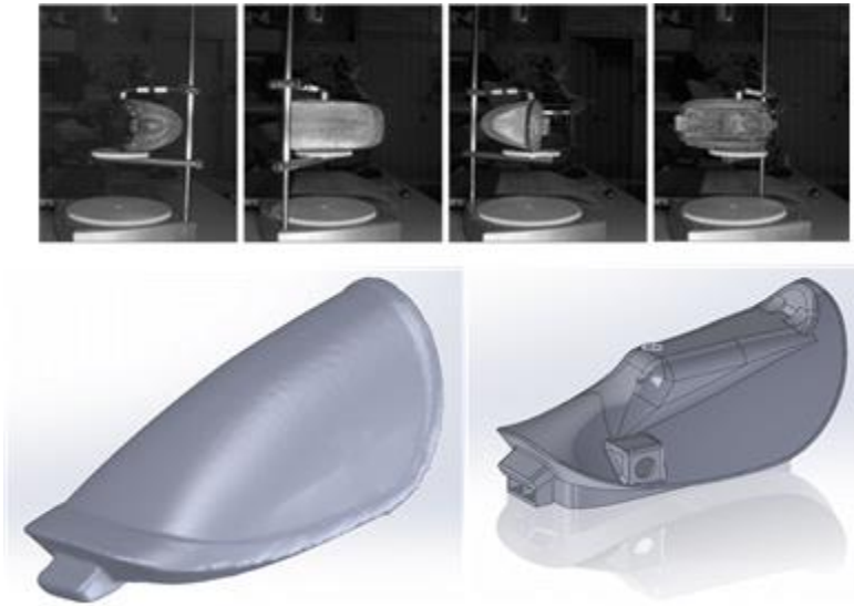
Fig. 5.3. Head Mount by 3d Scanning
