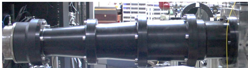
Figure 2.6 Contoured nozzle installed at AST-1 shock tunnel.
