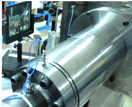
Figure 2.4 Conical nozzle installed at AST-1 shock tunnel.
