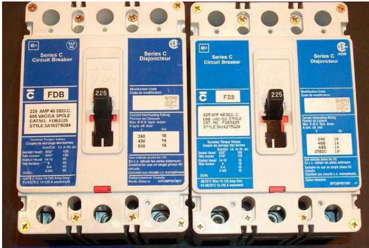
Figure 2.1.5 Counterfeit (left) and legitimate breaker (right) supplied to hospital in Montreal (courtesy CSA Group Inc.) (Geralde, 2010)
