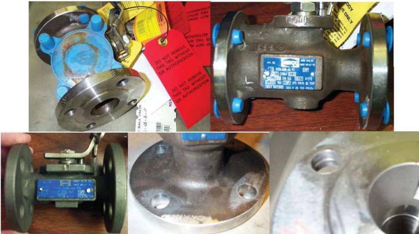
Figure 2.1.6 Flanges received as “new” at Savannah River - note clamp marks, different rivet sizes clamp marks, different rivet sizes (DOE, 2007)
