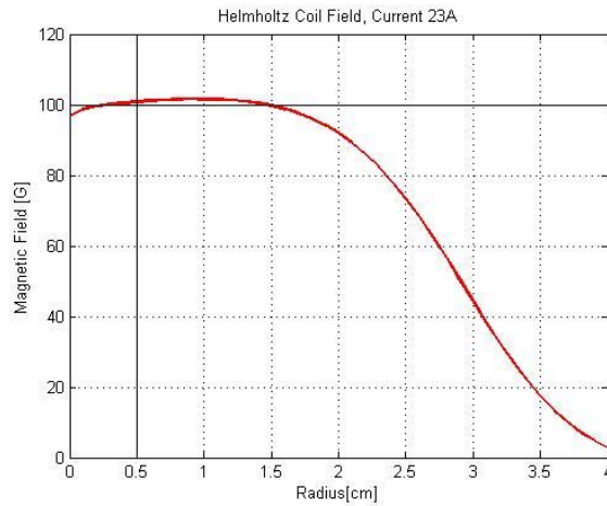
Figure 4.2 Calculated magnetic field generated in a Helmholtz coil. Solid lines mark the 100 G and 0.5 cm.
