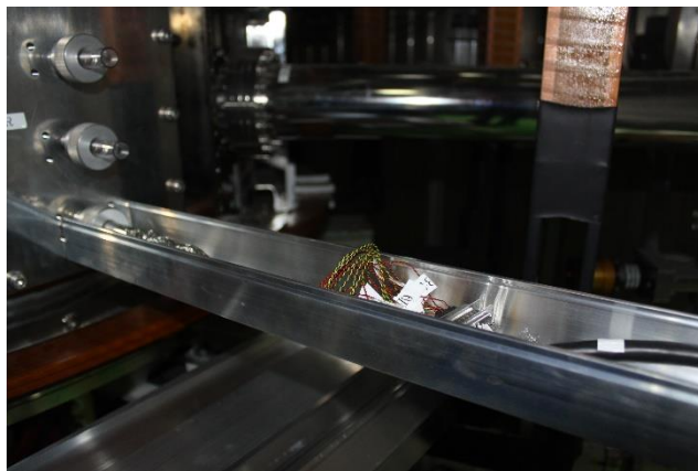
Figure 5.3 Image of internal magnetic probe array being installed, seen from the outside of the vacuum vessel.
