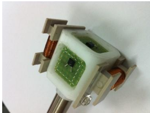
Figure 5.8 Image of the prototype of the internal magnetic probe array.
