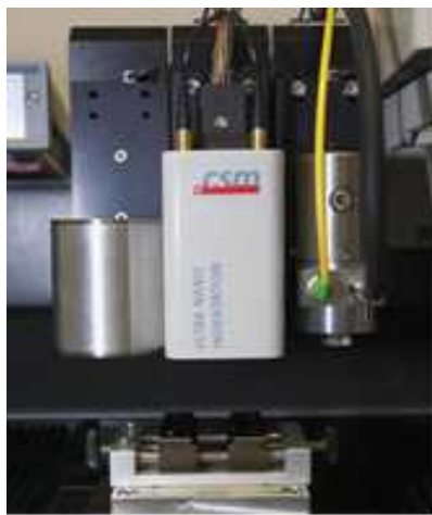
Figure 5.1 Nano indentation instrument & Berkovich indenter
