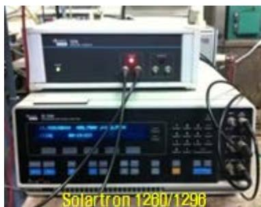
Fig. 3. 22. Impedance equipment (Solartron 1260/1296)
