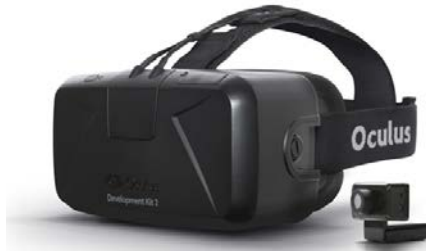
Figure 4-2 Oculus Rift Development Kit 2 and positional tracking
