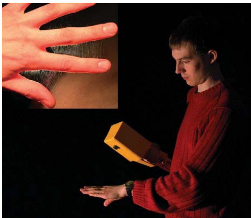
Figure II- 36. Handheld device for the electrospinning of wound dressings. Inset: PEO fibers electrospun from aqueous solution onto a hand (Manefield et al., 1999)
