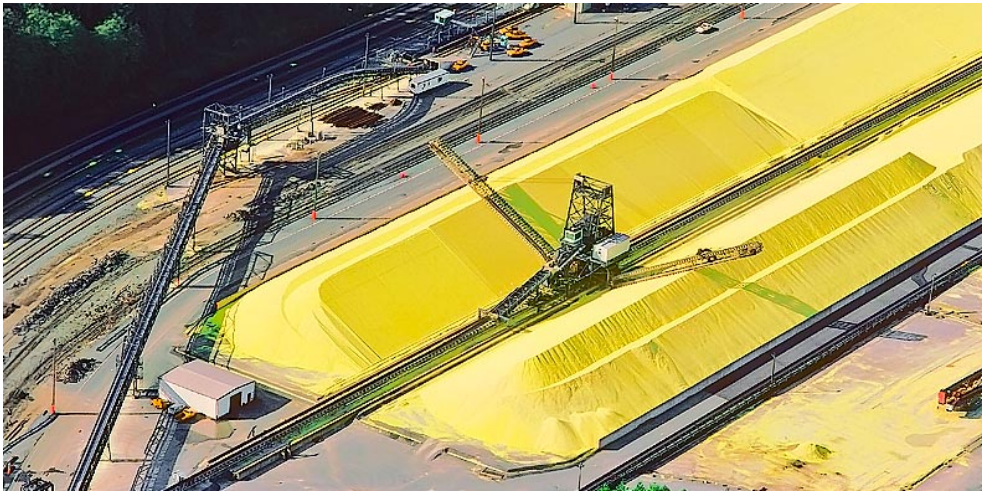
Figure 1.1 Example of an exposed deposit of elemental sulfur from hydrodesulfurization in petroleum refining processes.
