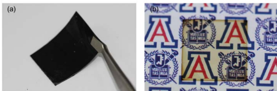
Figure 3.16 Photo images of PbS/poly(OLA-r-S) nanocomposite films: (a) A free-standing film prepared by solvent evaporation (film thickness = 1 mm). (b) A spin-cast film on a glass substrate (film thickness = 600 nm).
