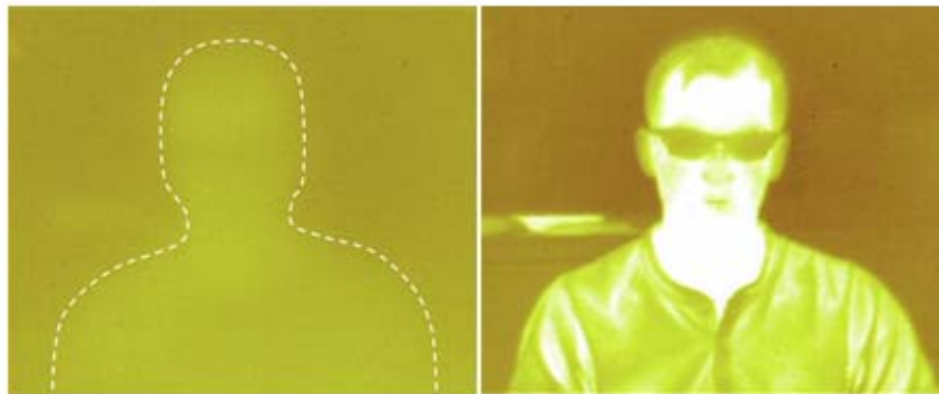
Figure 2.11 (top) IR Transmission spectra of PMMA and SDIB (20 wt%) copolymer lens. (left) A picture taken from IR camera with PMMA lens. (right) A picture taken from IR camera with SDIB copolymer (20 wt%) lens.
