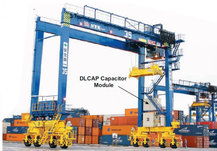
Figure 1-8. Hybrid diesel/electric rubber-tired gantry crane with DLCAP electrochemical capacitor energy storage system (fuel saving of 40 % are typical). Adapted from J. R. Miller et al [74].
