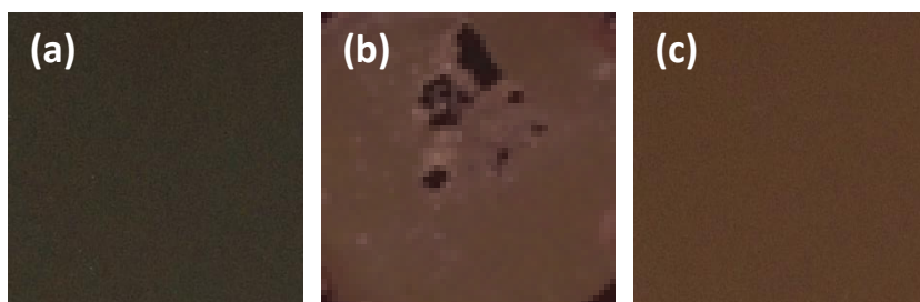
Figure 4.11. Pictures of (a) as-prepared NiWP film and (b, c) Cu film electrodeposited (b) without coulometric reduction process or (c) after coulometric process on NiWP film.
