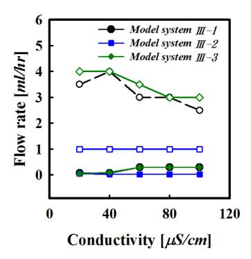
**Figure 5.11.** Flow rate range for Taylor cone jet formation as a function of electrical conductivity for model systems Ⅲ-1, 2, and 3; filled symbols for the initial and open symbols for the final flow rate
