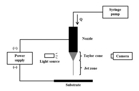
Figure 4.1. Schematics for the EHD jet printing experimental setup
