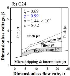
Figure 5.6. Processing window maps for Model system II: (a) C18, (b) C24.
