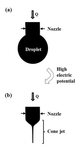
**Figure 2.1.** Schematic illustration of the cone-jet transition where electric potential induces the change of liquid shape from droplet to cone jet: (a) droplet shape with no electric potential, (b) conical shape with high electric potential.
