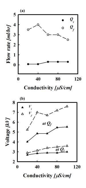
**Figure 5.10.** Flow rate range (a) and voltage range (b) of Taylor cone jet zone as a function of electrical conductivity for model system III-1
