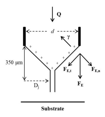
Figure 5.8. The schematic of force exerted on the surface of Taylor cone
