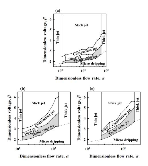
**Figure 5.13.** Processing window maps for model system Ⅲ-1: (a) M10K20, (b) M10K60, (c) M10K100.
