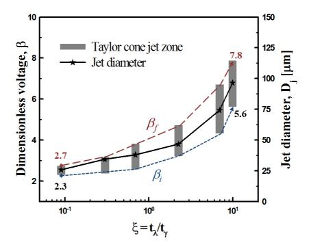
**Figure 5.5.** Range of the dimensionless voltage for Taylor cone jet and corresponding jet diameter as a function of  $\xi$
