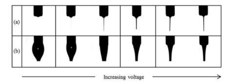
**Figure 5.2.** Evolution of cone jet of PEO ( $M_w = 1.0 \times 10^6 \ g/mol$ , 0.38 wt%) in W/G mixture: (a) thin jet from the insufficient flow rate, (b) thick jet from the excessive flow rate.
