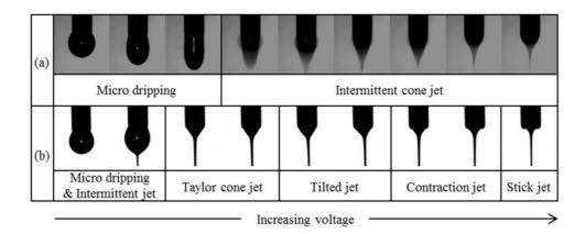
**Figure 5.1.** Evolution of cone jets: (a) W/G mixture (Newtonian fluid), (b) PEO ( $M_w = 1.0 \times 10^6 \ g/mol$ , 0.38 wt%) in W/G mixture (viscoelastic fluid).
