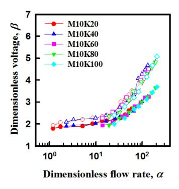
**Figure 5.14.** Model system Ⅲ-1. Dimensionless initial (filled symbol) and final voltage (open symbol) of Taylor cone jet formation as a function of dimensionless flow rate
