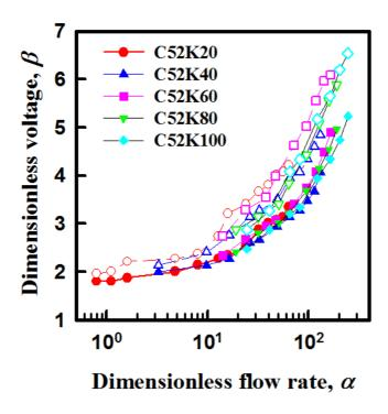
**Figure 5.16.** Model system Ⅲ-3. Dimensionless initial (filled symbol) and final voltage (open symbol) of Taylor cone jet formation as a function of dimensionless flow rate
