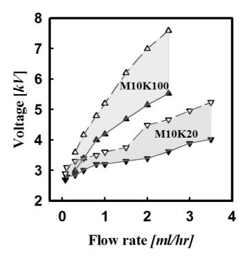
**Figure 5.9.** Processing conditions (gray regions) of Taylor cone jet for PEO solutions with different electrical conductivity; filled triangles for initial voltage  $(V_i)$  and open triangles for the final voltage  $(V_f)$ .
