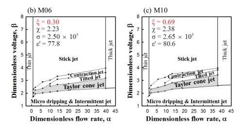
**Figure 5.3.** Processing window maps for model system I with different elasticity: (a) M03, (b) M06, (c) M10.
