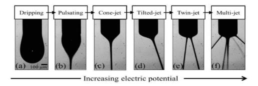
**Figure 2.2.** Electrohydrodynamic jetting modes with respect to electric potential [Lee et al. (2013)]
