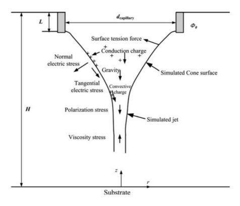
**Figure 2.3.** The schematic of electrode configuration and force exerted on the cone-jet [Wei et al. (2013)]
