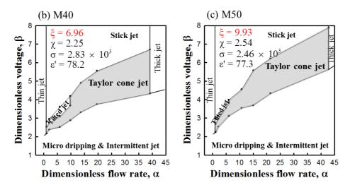
**Figure 5.4.** Processing window maps for model system I with different elasticity: (a) M20, (b) M40, (c) M50.
