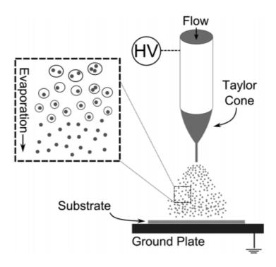
**Figure 2.5.** Electrospray of colloidal dispersion. The high electric potential deforms fluid at the edge of the capillary tube in to a Taylor cone. A jet emits from the apex of the cone and breaks up in to charged droplets. The droplets rapidly evaporate, leaving dry material that is deposited on to the substrate [Brown et al. (2015)].
