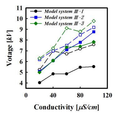
**Figure 5.12.** Voltage range at final flow rate for Taylor cone jet formation as a function of electrical conductivity for model systems III-1, 2, and 3; filled symbols for the initial and open symbols for the final voltage
