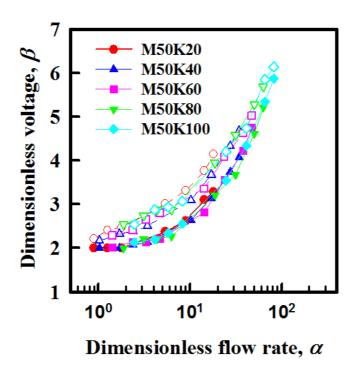
**Figure 5.15.** Model system Ⅲ-2. Dimensionless initial (filled symbol) and final voltage (open symbol) of Taylor cone jet formation as a function of dimensionless flow rate
