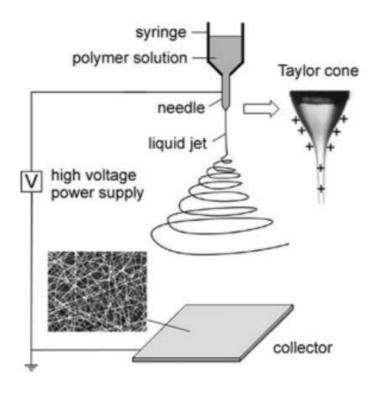
**Figure 2.4.** Schematic illustration of the basic setup for electrospinning. The insets show a drawing of the electrified Taylor cone and a typical SEM image of the nonwoven mat of poly(vinyl pyrrolidone) (PVP) nanofiber deposited on the collector [Li et al. (2004)].
