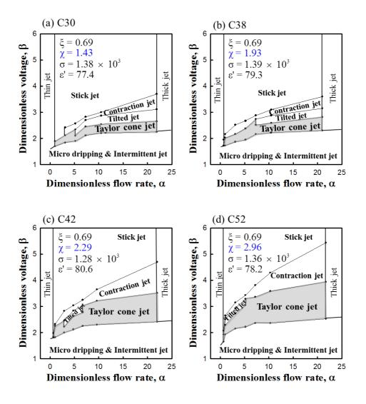
**Figure 5.7.** Processing window maps for Model system Ⅱ: (a) C30, (b) C38, (c) C42, (d) C52.
