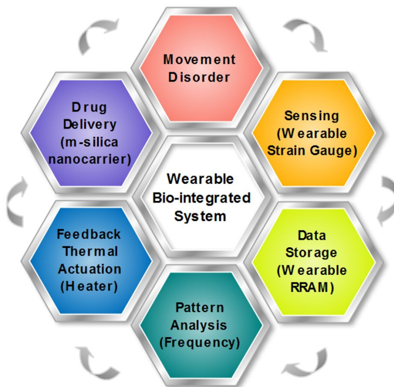
Figure 2.12 Schematic illustration of the operation process of the wearable bio-integrated system: wearable strain sensor detects movement disorders, the recorded data are stored in onboard memory modules, diagnostic patterns are analyzed on the basis of the stored data stream, thermal actuators apply heat to drug-loaded m-silica NPs, drugs are diffused transdermally, and movement disorders can be treated.
