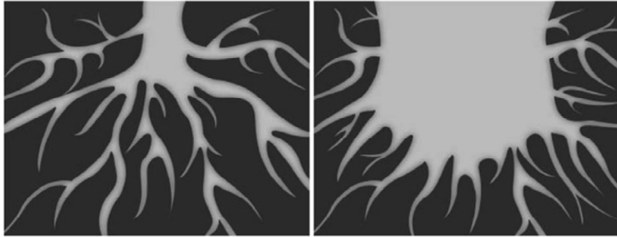
Figure 4-16. Schematics showing the pore characteristics of a typical microporous carbon material (left) and a hierarchically porous MDC-D (right).
