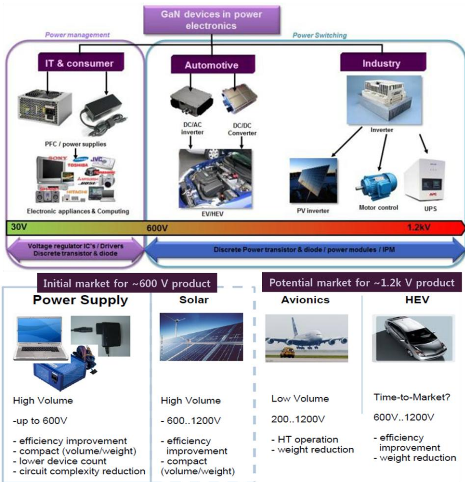
Figure 1.10 Fields of applications for GaN power devices and target applications of commercial GaN products.
