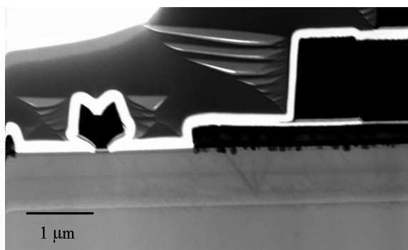
Figure 2.28 (a) Structure of the AlGaIn/GaN HEMT with field plate, (b) comparison of electric field for the HEMT with field plate and normal HEMT, (c) Microscope image of HEMT with field plate.
