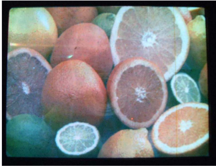
Figure 1-2 Four-inch QVGA bottom-emission AMOLED display driven by oxide TFTs without any pixel compensation circuit. [27]
