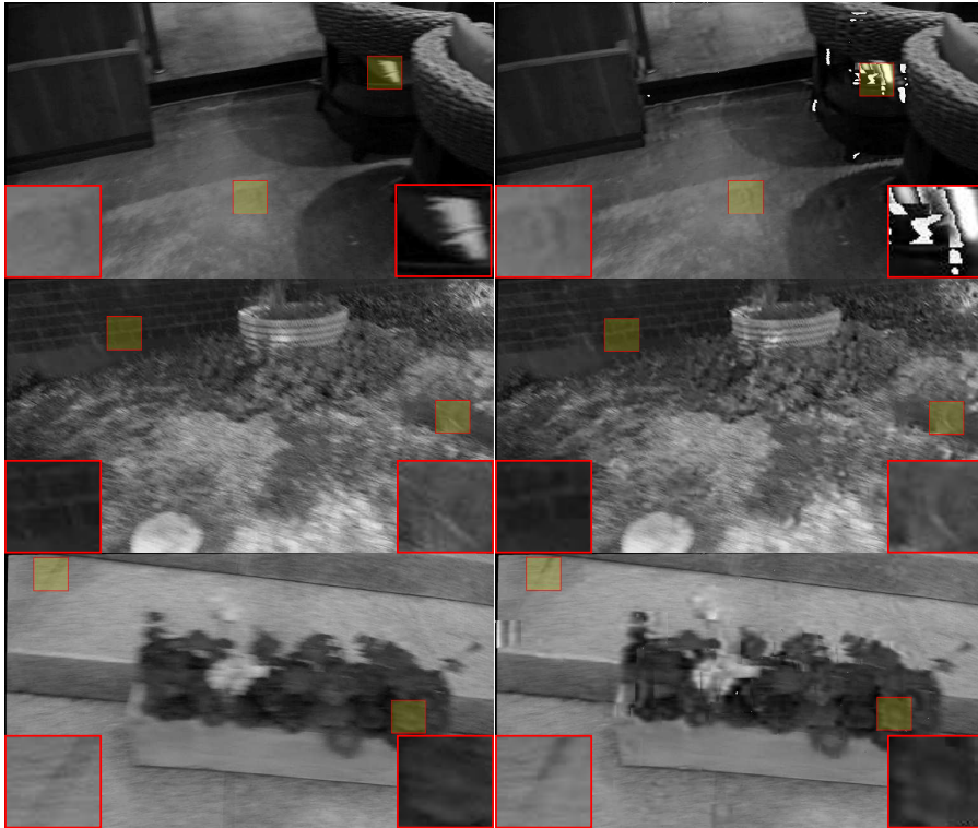
Figure 7.7: Deblurring results are visualized for each dataset. From top to row, the images are from cafe , statue , and flowers sequence. From left to right, the original images and the corresponding deblurred images are shown. The red boxes with yellow masks are magnified in the bottom corners of each image. Note that the right red box of the cafe dataset shows the failure case where the presence of disparity discontinuities made some undesired visual artifacts.
