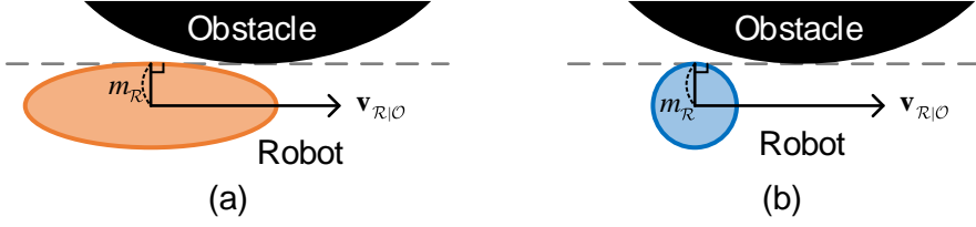
Figure 4.10 A basic concept of determining preferred angular velocities. (a) An elliptic robot whose orientation is aligned with \mathbf{v}_{\mathcal{R}|\mathcal{O}} can avoid obstacles with the same path as (b) a circular robot with radius equal to minor radius of the elliptic one does.
