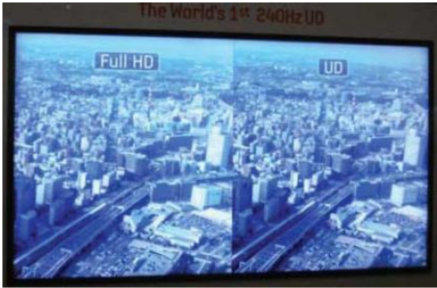
Figure 2.2 Prototype 70" IGZO ultra definition LCD TV (Ref. DisplaySearch)
