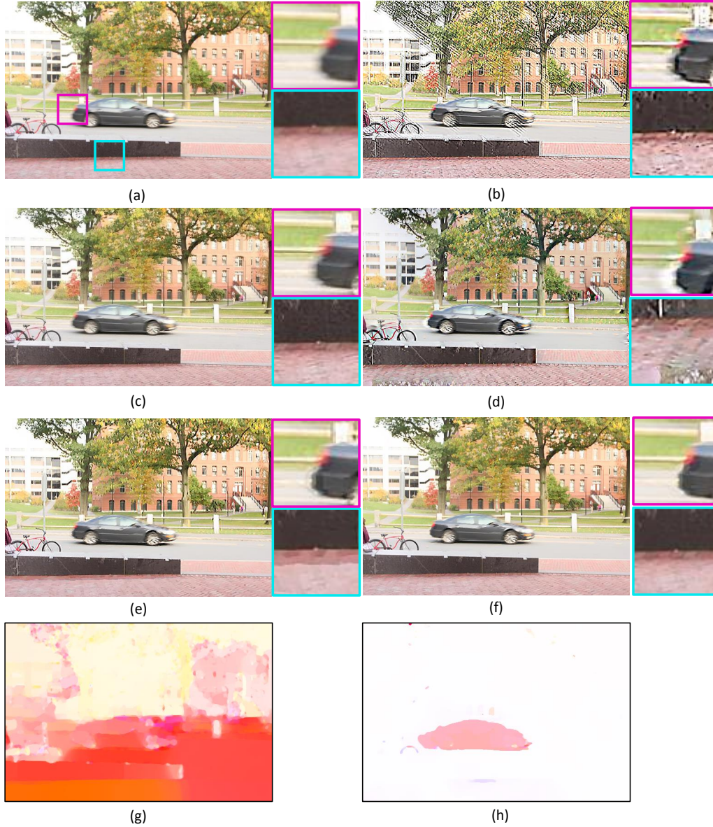
Figure 4.4: Qualitative comparisons. (a) Real Blurry image. (b) Result from [13]. (c) Result from [6]. (d) Result from our segmentation-based method [10]. (e) Deblurring result without motion cues. (f) Deblurring result with motion cues. (g) Flow result without using motion cues. (h) Flow result with motion cues.
