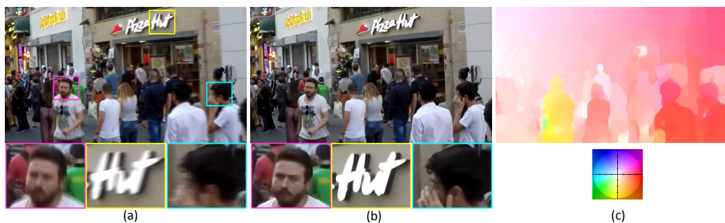
Figure 5.1: (a) A blurry frame in a dynamic scene. (b) Our deblurring result. (c) Our color coded optical flow estimation result.
