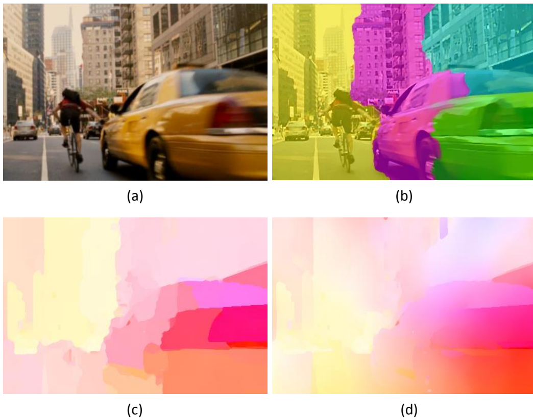
Figure 4.5: Robust regularization. (a) Real blurry image. (b) Segmentation result from our segmentation-based deblurring method [10]. (c) Motion flow with TV regularization ( \mathbf{v} = 0 ). (d) Motion flow with our TGV regularization.
