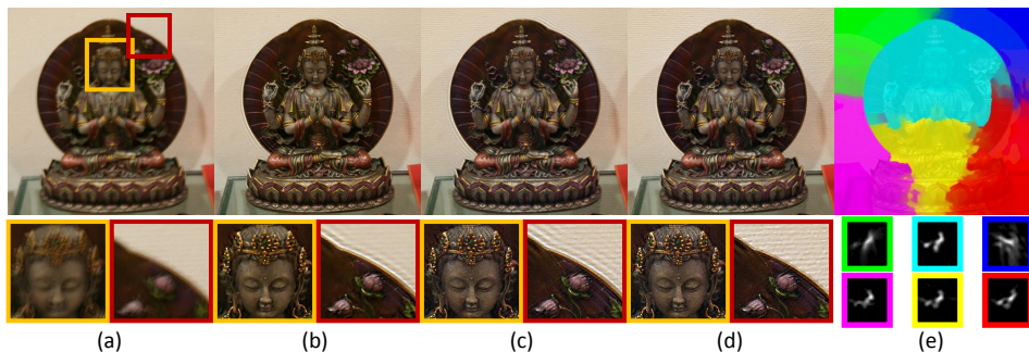
Figure 2.2: Multiple blur kernel models give a much better result without additional process to remove ringing artifact. (a) A blurry image of static scene. (b) Deblurring result of Shan et al. [3]. (c) Our deblurring result with one uniform kernel. (d) Our segmentation-based deblurring result. (e) Illustration of six weight variables. Slightly different blur kernels are estimated.
