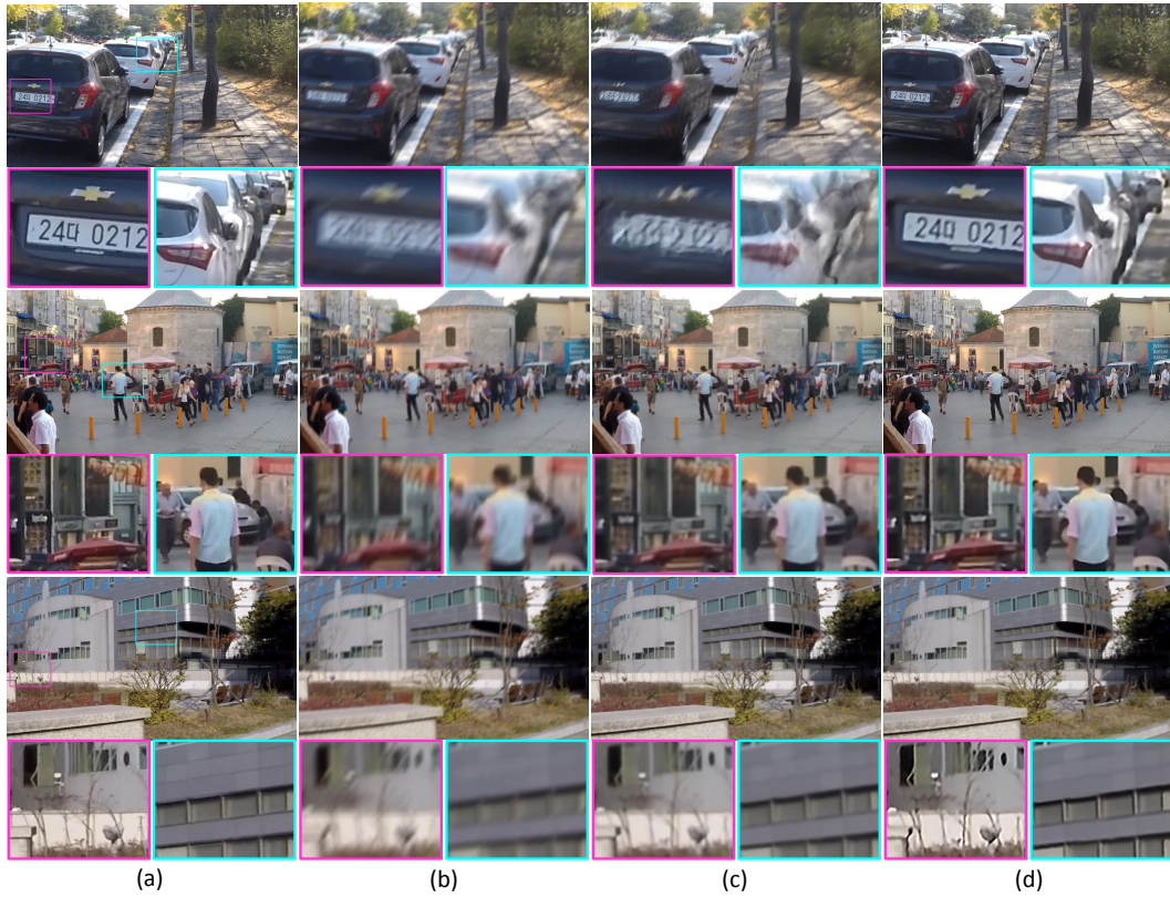
Figure 5.13: Comparative deblurring results using our blur dataset. (a) Ground truth sharp frames. (b) Generated blurry frames including both motion and defocus blurs. (c) Deblurring results from without handling defocus blurs. (d) Deblurring results handling defocus blurs.
