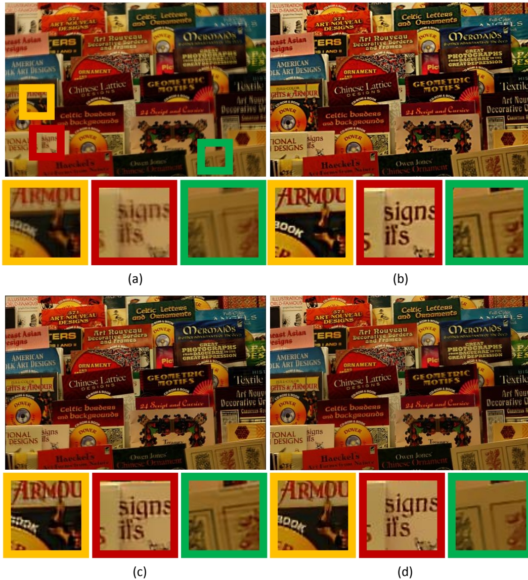
Figure 2.8: Comparison of static scene deblurring. Magazine image is blurred by rotational camera shake and requires non-uniform blur kernel to be restored. (a) Blurry Magazine image. (b) Result of Hirsch et al. [4]. (c) Result of Gupta et al. [5]. (d) Our segmentation-based deblurring result.
