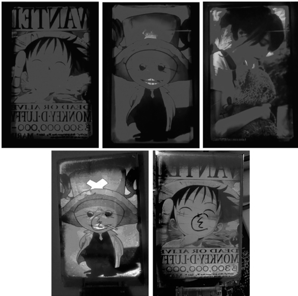
Figure 1.3 Display image of 4.3-inch red and green QLED using a LTPS TFT backplane with a 480 \times 800 pixel array for the active matrix drive. [15] (The image is taken from ref. [15])
