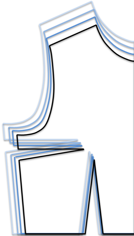
Figure 1.1 Linear grading of bodice panel. Linear grading method performs the grading job by applying translations to a set of panel vertices according to predetermined directions.
