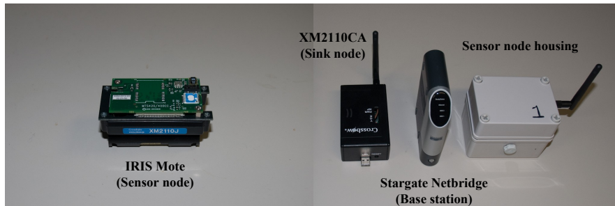
Figure 2.2 Components of a WSN for wildfire monitoring system.
