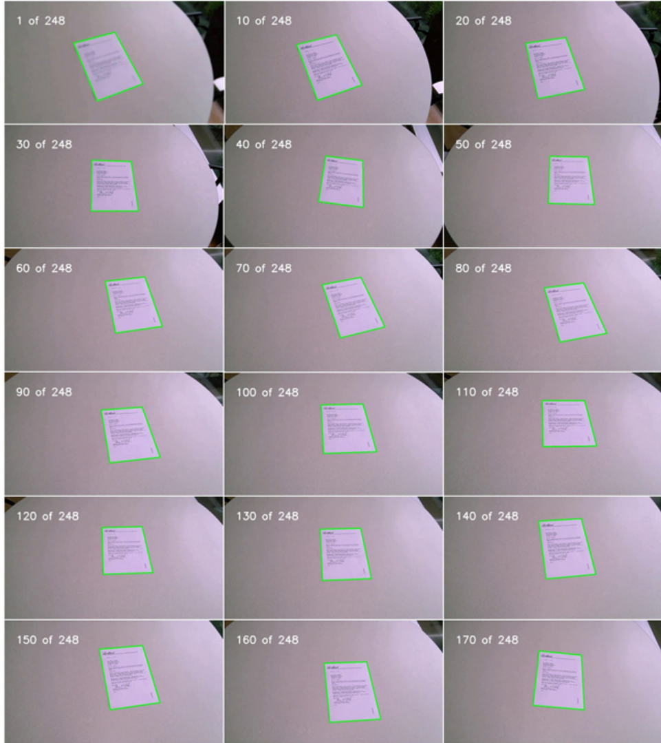
Figure 4.9: Results of the proposed method for a letter video in Background 2 . The green solid contour is the detected boundaries and frame number is indicated at top-left side (The format is ‘ t of total frame number’).
