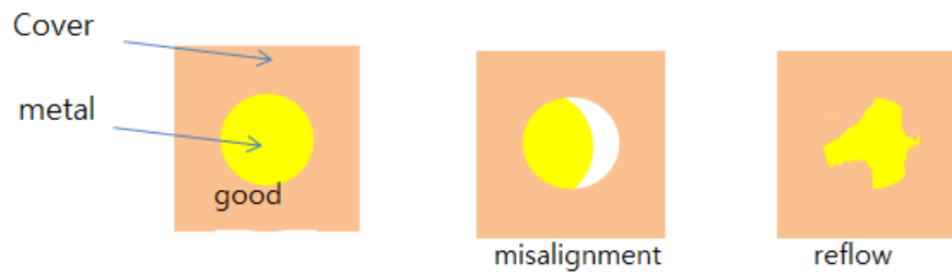
Figure 2-4 Problems associated with the previous method laminating a cover layer with pre-drilled holes: misalignment and cover layer reflow.
