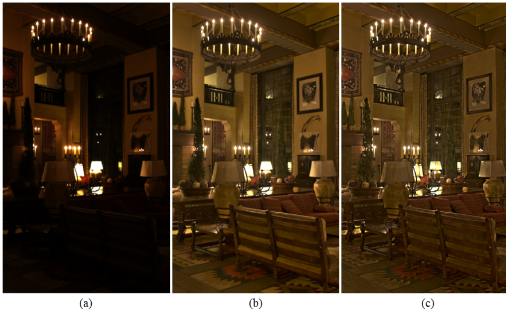
Figure 4.8: HDR tone mapping result 3 (a) original image (b) WLS (c) proposed method
