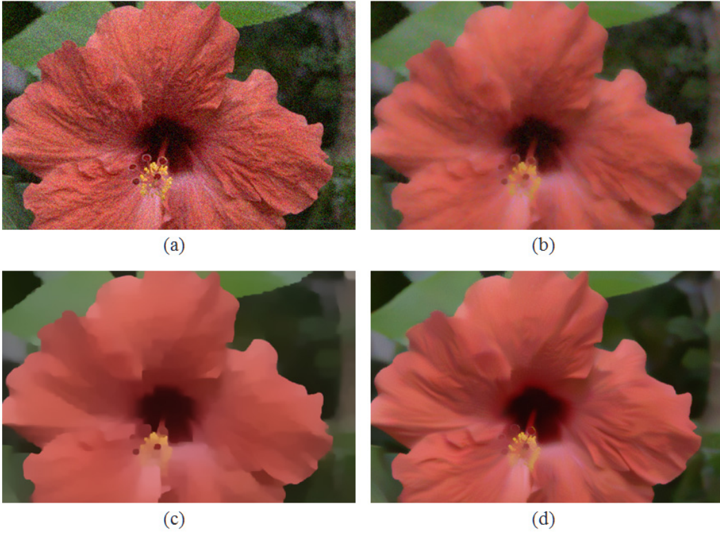
Figure 4.13: Edge-preserving smoothing of noisy image (a) noisy image (b) WLS [1] (c) RTV [2] (d) proposed
