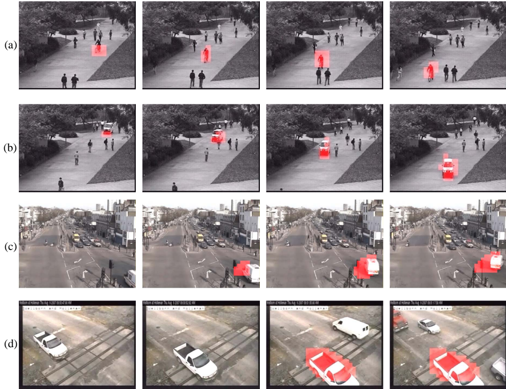
Figure 4.13 Examples of anomaly detections related to the second requirement (Speed information). (a,b) over speed on a pavement; (c) going on the opposite direction; (d) a car stops on a railway. (best viewed in color)
