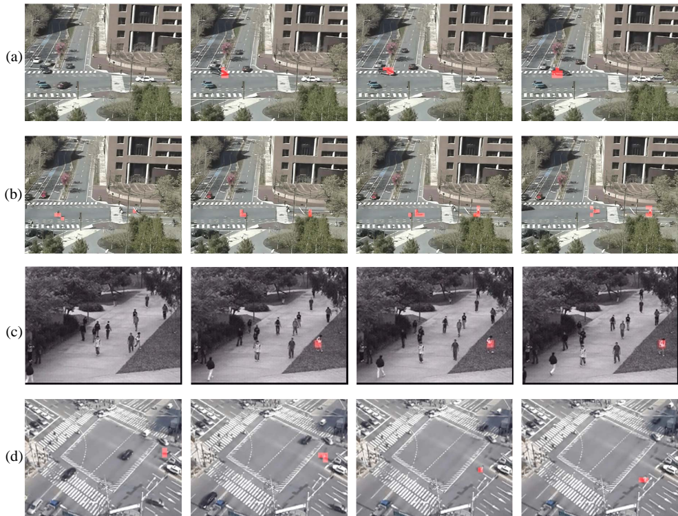
Figure 4.12 Examples of anomaly detections related to the first requirement (semantic regions of normal pattern). (a) illegal U-turn; (b) jaywalking; (c) intrusion of restricted areas; (d) driving on the wrong direction. (best viewed in color)
