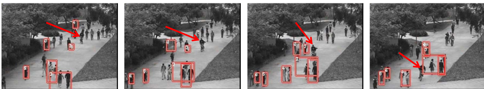
Figure 4.18 Tracking failure case of the object based multi-target tracking method in a crowded scene. (best viewed in color)
