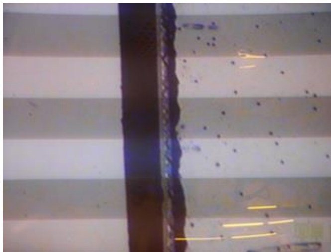
Fig. 4.15. Microscope picture of before (left) and after (right) selective wet etching.
