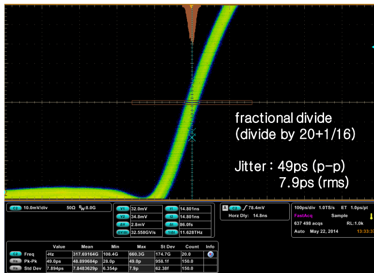
Fig. 5.21 Measured jitter with division number 20+1/16 (fractional).
