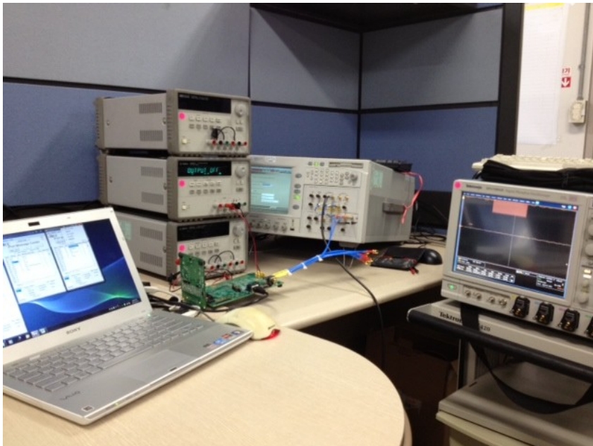
Fig. 3.21 Test environment for the fabricated chip..
