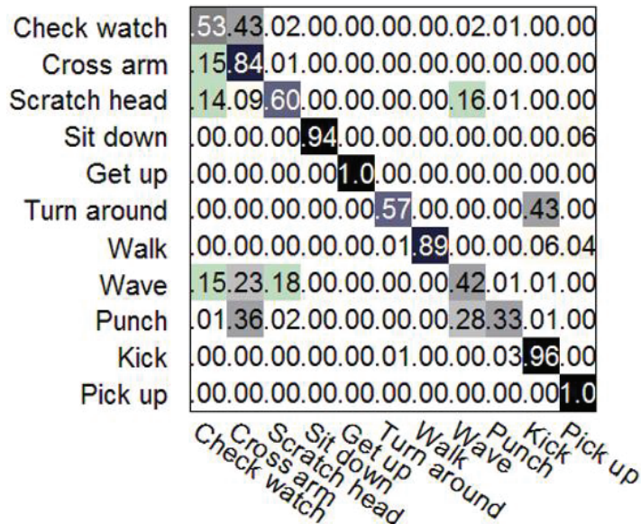
Figure 3.27: Confusion matrix of SNU dataset. The confusion matrix when we train using IXMAS dataset and test using SNU dataset.
