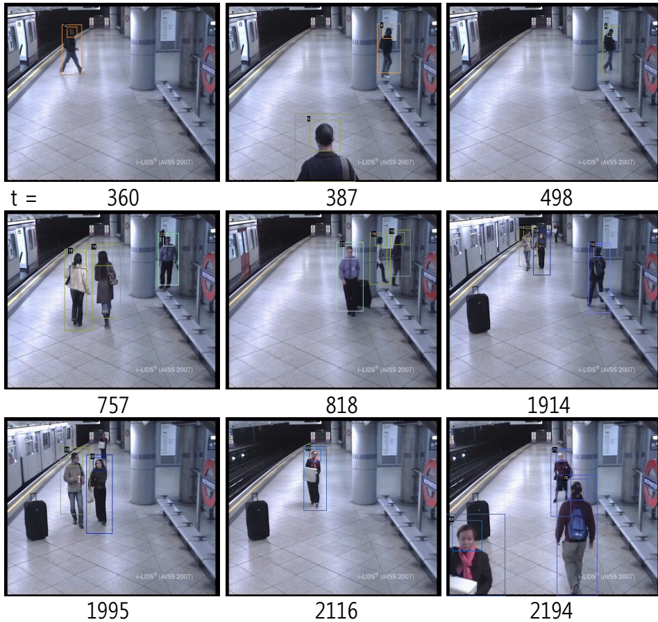
Figure 2.9: The qualitative results for the iLids 2007 AVSS dataset. The squares are detected heads and the rectangles are estimated body of each person.
