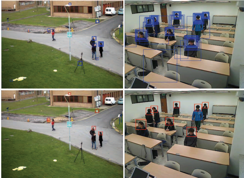
Figure 2.3: Upper row: Row head detection results by [51]. Bottom row: Filtered head detection result by the outlier rejection and the meanshift clustering algorithm. The proposed data association method is processed with these filtered boxes.
