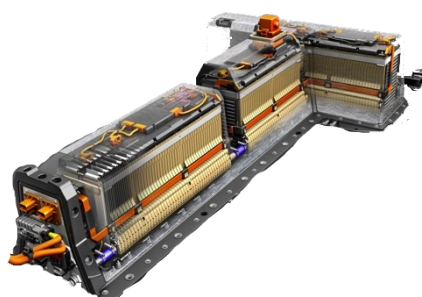
(a) Chevy Volt battery system (16.5 kWh, Li-ion)
