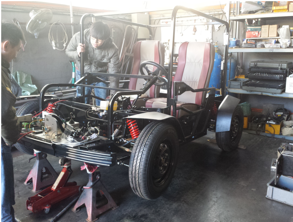
Figure 6.1 Prototype EV frame with traction motors, steering and suspension system assembled.
