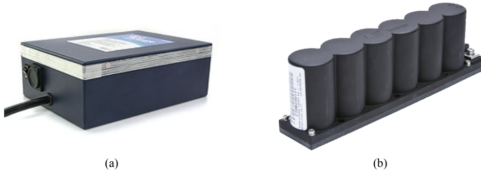
Figure 6.3 HESS storage elements. (a) Li-polymer battery pack 24 V/20 Ah. (b) Supercapacitor module 58 F/16.8 V from LS Mtron.
