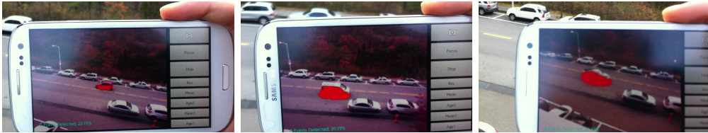
Figure 2.8: Example detection results of our method on a mobile device (foreground pixels highlighted in red). Our implementation runs approximately 20 frames per second, assuring real-time performance.
