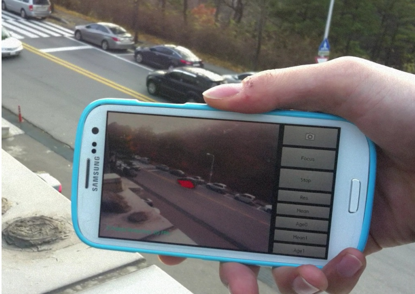
Figure 2.1: Example of our method running on a mobile device (foreground pixels highlighted in red). Our implementation runs approximately 20 frames per second, comfortably in real-time.
