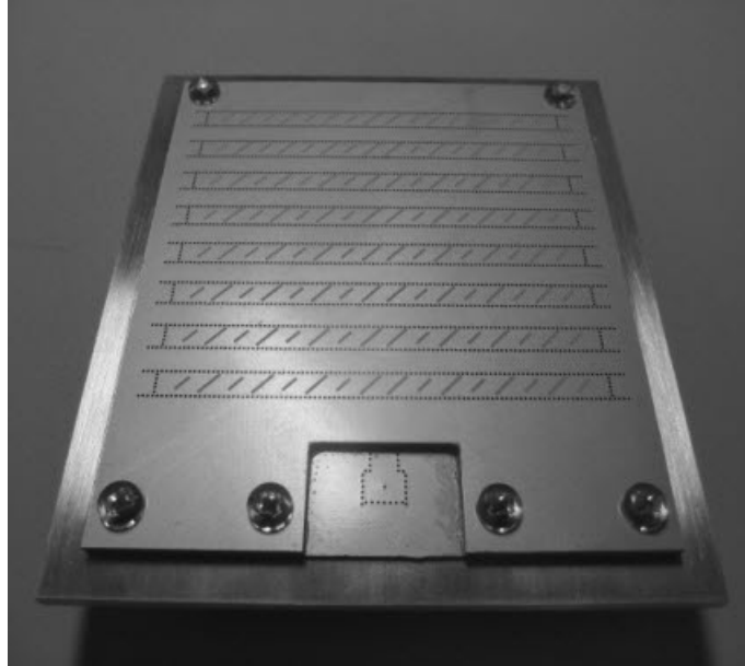
Fig. 3.15 The fabricated slot array antenna for 45°-inclined LP.
