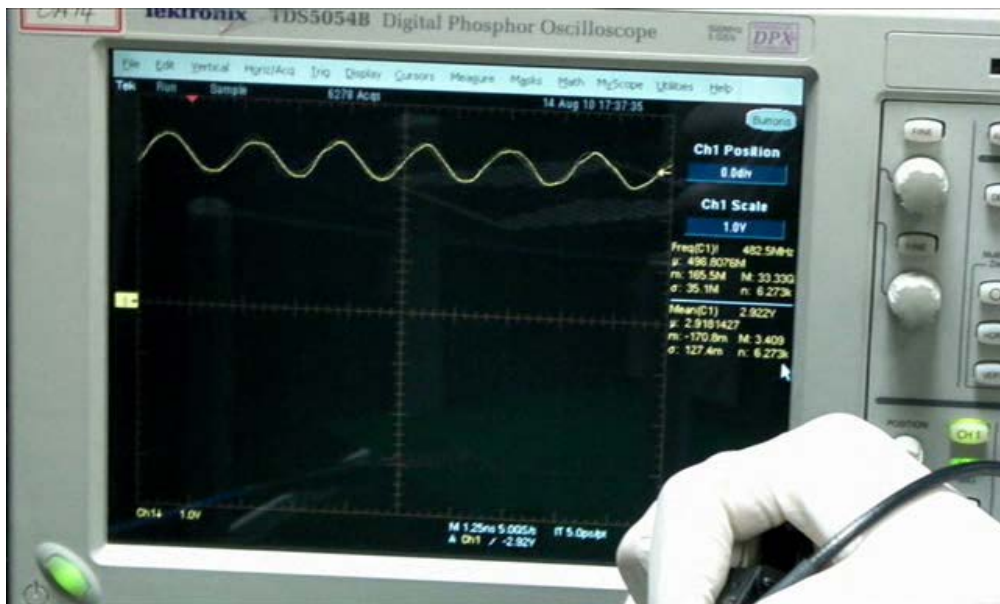
Figure 4.20 Rectifying signal of 500 MHz operable rectifier with antenna.
