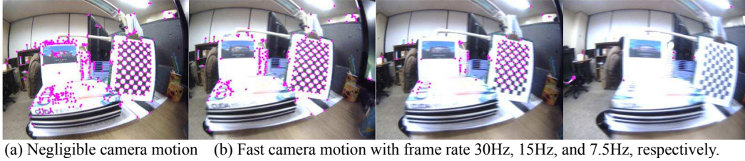
Figure 2.1: Motion blurs and detected Harris corner points [1] with different frame rates. (a) Negligible camera motion with frame rate of 15Hz for a comparison. (b) Fast camera motion with frame rate of 30Hz, 15Hz, and 7.5Hz, respectively. As motion blur becomes severer by decreasing frame rate, the number of detected corner points rapidly decreases.
