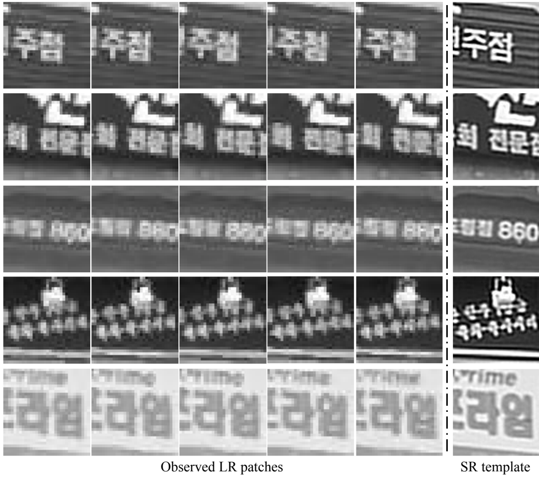
Figure 3.7: Super-resolution results for building sequence. Left: Low-resolution patches tracked in input images. Right: Super-resolution patches ( \times 3 ) by the proposed method.
