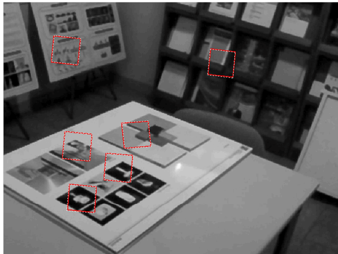
Figure 3.5: Projected landmarks after camera pose estimation (white dotted lines) and observed landmarks (red solid rectangles), which indicate the accuracy of SLAM results indirectly.
