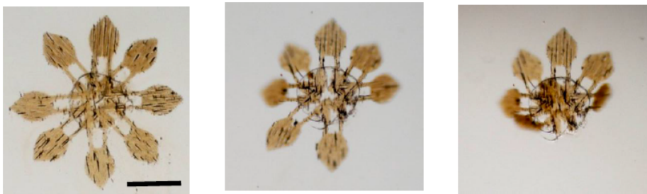
Figure 4.9 Blooming flower-like actuator on circularly patterned PDMS. When the magnetic field is applied perpendicular to the substrate surface, the flower closes in on itself, bending its eight identical petals. (Scale bar: 500 \mu m)
