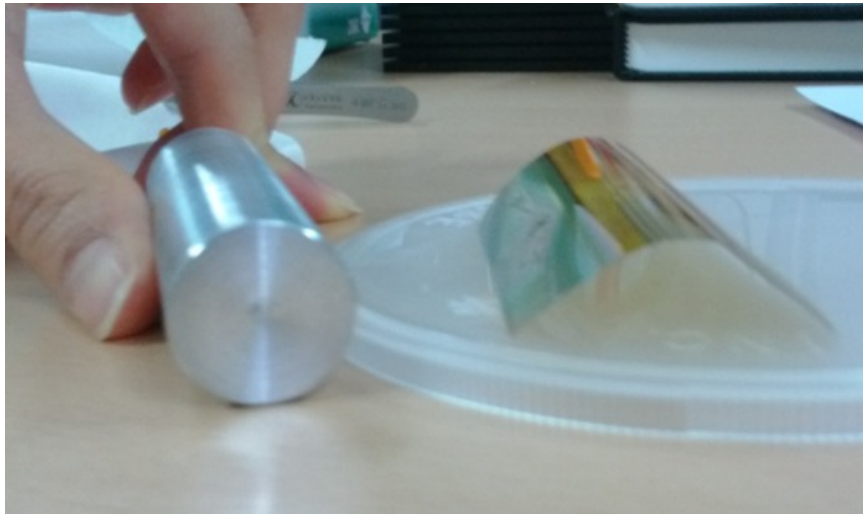
Figure 5.9 Flexible IGZO TFT sample and 10 mm bending chuck.
