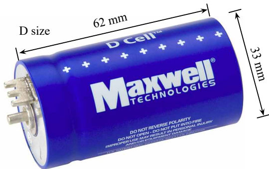
Maxwell Technologies BCAP0310 Capacitance: 310 F Rated voltage: 2.7 V Rated capacity: 0.31 Wh
