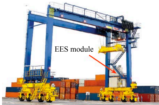
(a) Regenerative energy storage for a seaport crane
