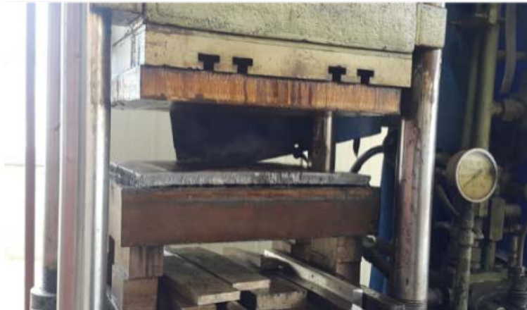
Figure 3.21 Cutting and flattening of the specimen for the tension test
