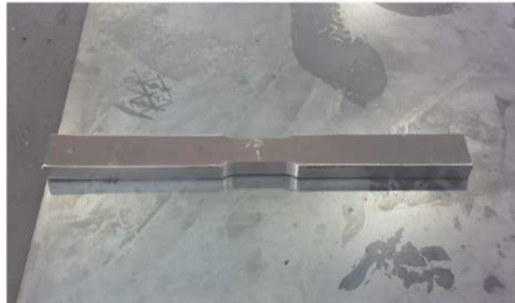
Figure 3.21 Cutting and flattening of the specimen for the tension test
