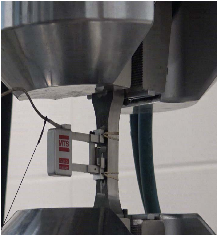
Figure 3.4 Uniaxial cyclic loading test on X70 specimen
