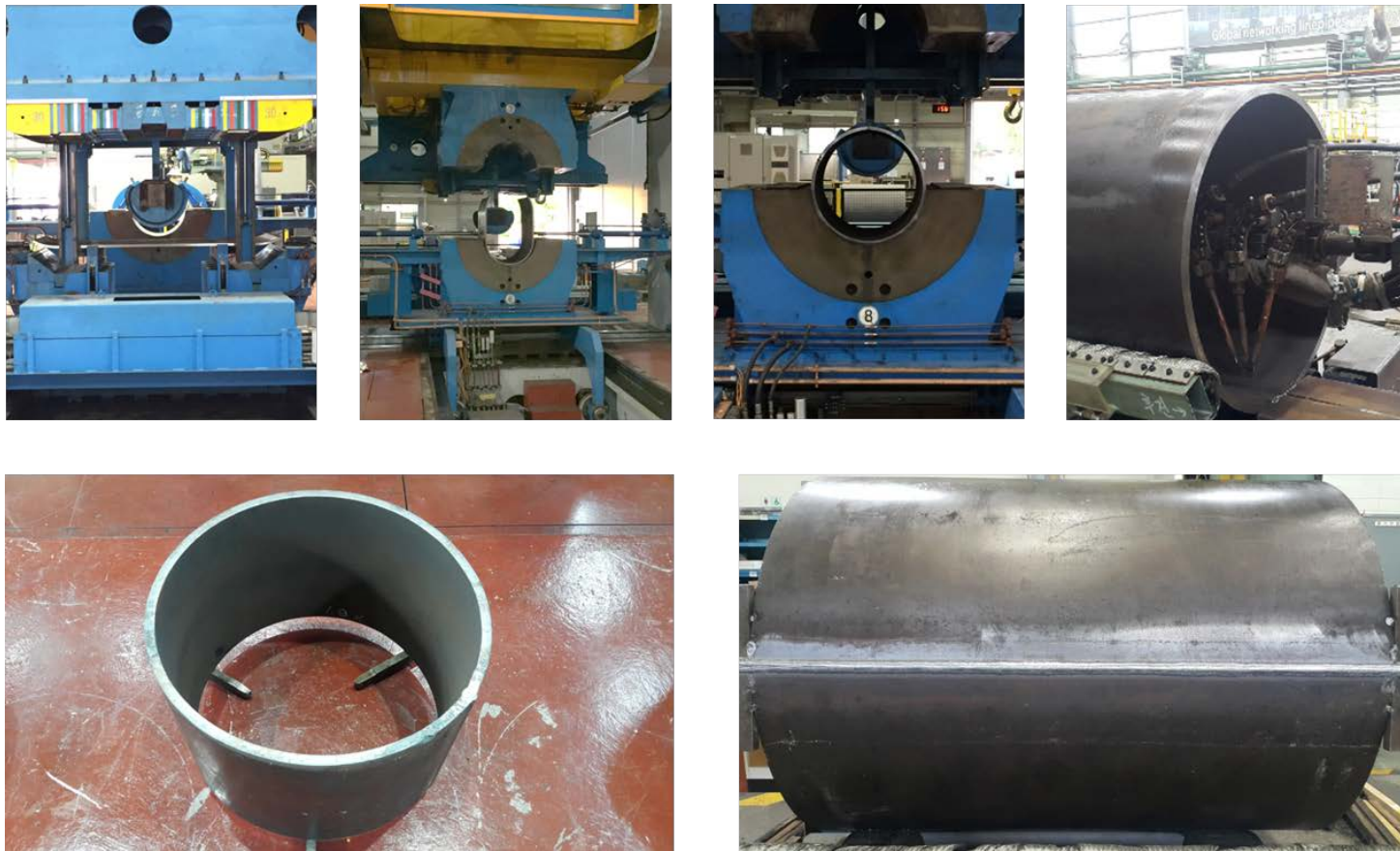
Figure 3.17 Experimental test of the UOE pipe forming
