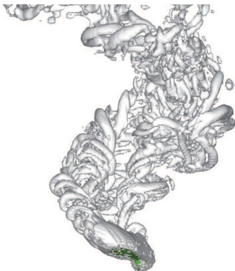
Figure 3.14. Vortical structures around the seed model at four different time instants, identified by the isosurface of \lambda_2 = -0.1 : (a) tu_g/c = 138 ; (b) 334; (c) 402; (d) 4000. The seed model is colored in green.
