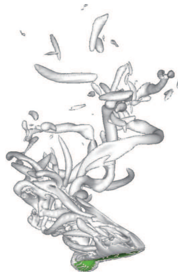
Figure 3.14. Vortical structures around the seed model at four different time instants, identified by the isosurface of \lambda_2 = -0.1 : (a) tu_g/c = 138 ; (b) 334; (c) 402; (d) 4000. The seed model is colored in green.
