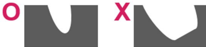
Figure 4.20 Tendency of fabricated groove according to number of scanning and resulted shape of tilted groove according to bottom width
