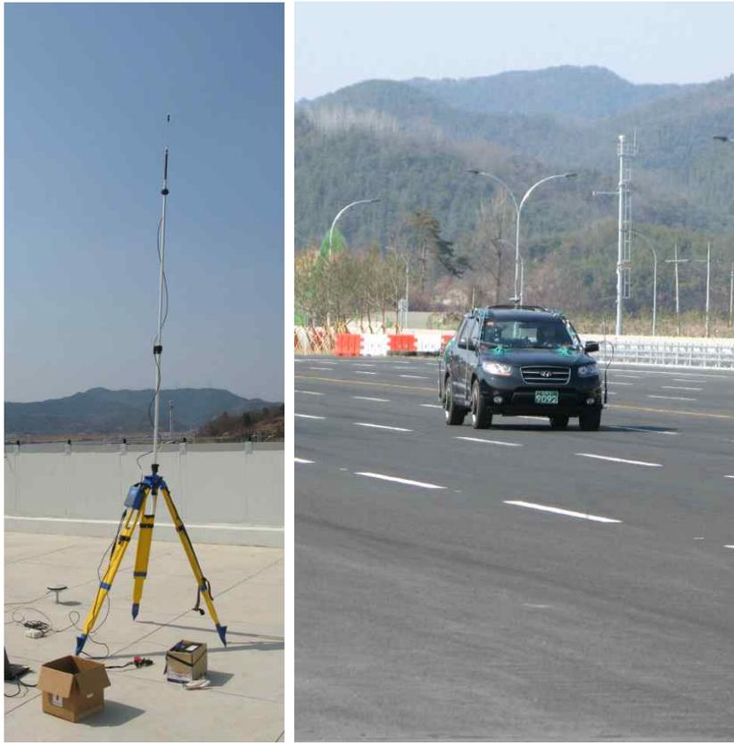
Figure 4.9 GPS/RTK for measuring exact vehicle speed and position(Base on left figure, equipped test vehicle on right figure)
