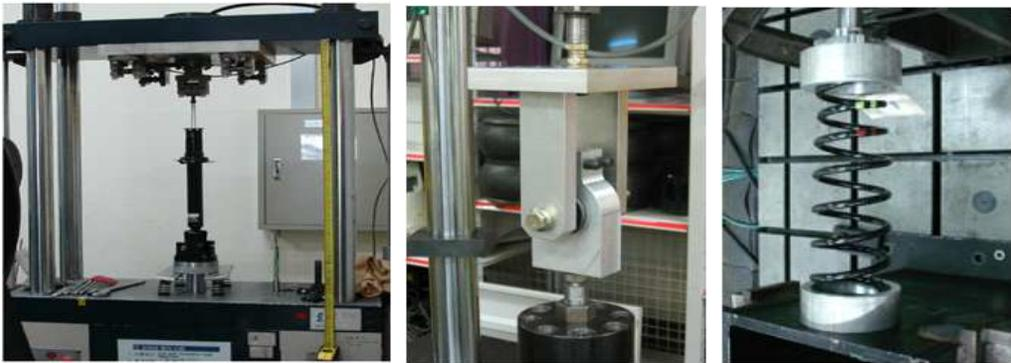
Figure A3. Suspension components test(from left : damper, bush, spring)
