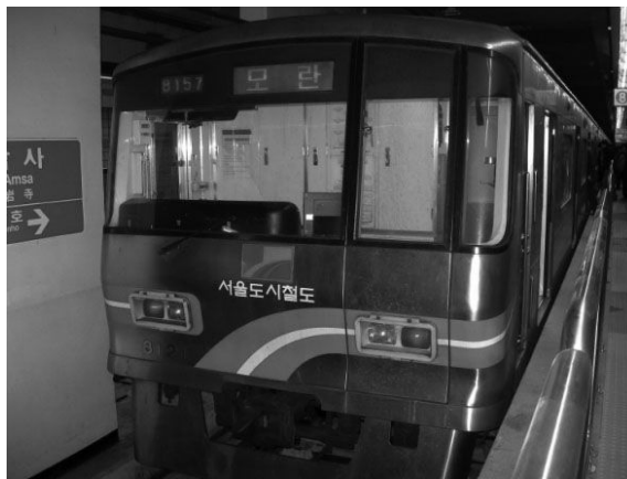
Fig. 20 Train blunt nose shape of Seoul Subway Line 8
