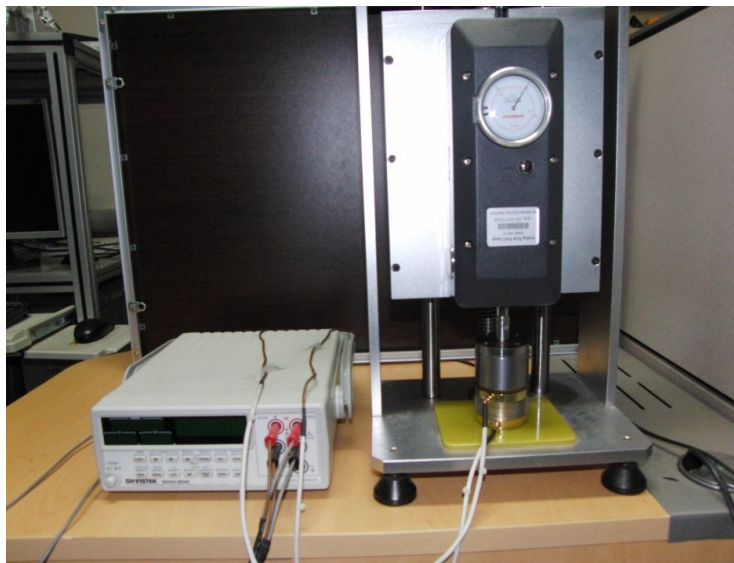
Fig. 3.15 Experimental setup for measuring electric resistances of BPs.
